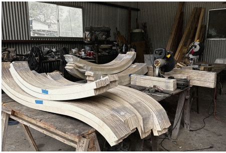
The ribs in the shop: laminated birch, bent to the drawing on a jig made for each curve.
